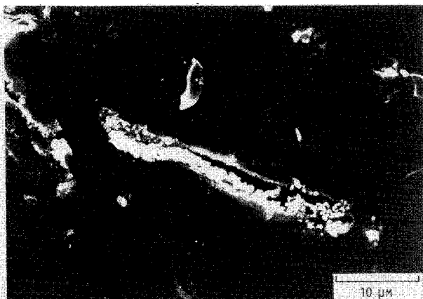
Fig. 7 Surface of a sample identical to that of Fig. 5 after 90 h of plasma asher exposure. Oxidative undercutting around the elongated defect is clearly visible.
